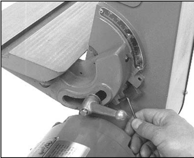
Figure 10. Adjusting belt table stops.
